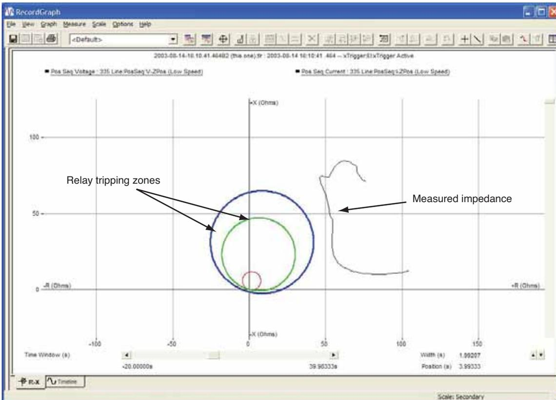
Power swing impedance vs. relay tripping zones
