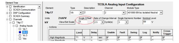
Users must manually correct the angle measurement by comparing the applied signal's phase angle to the metering screen displayed angle. This Angle Offset setting is used to adjust the angle error due to the measurement until the angle in the metering screen matches with the applied signal's phase angle.
