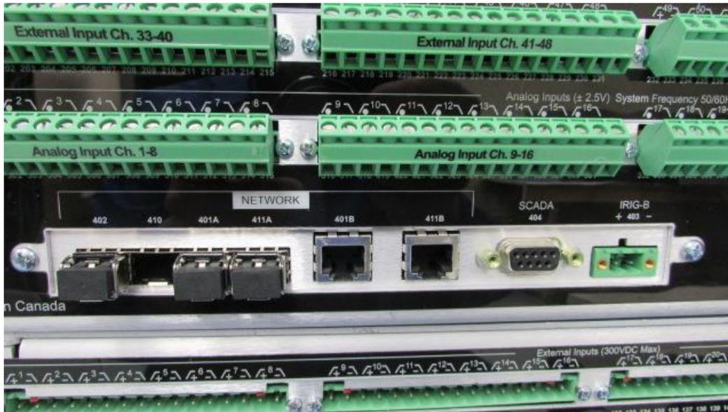
**Figure 2 – Rear view of a TESLA 4000 with redundant network ports**
