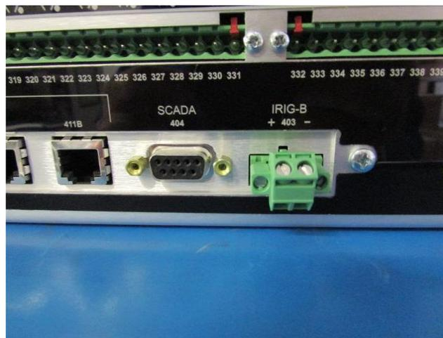
**Figure 4 - IRIG-B and SCADA RS-232 ports**
