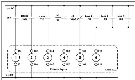
Contact trigger DC schematic
