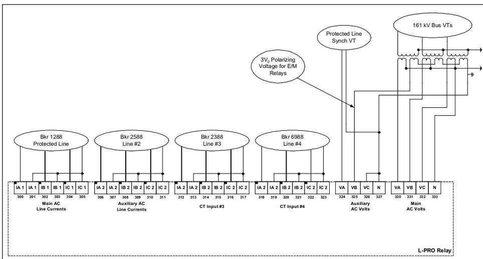
Analog channel input connections
