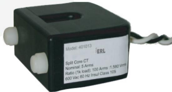
The split core transformer measures current in a 5 A or 1 A secondary CT circuit and works in conjunction with the TESLA disturbance fault recorder to monitor secondary currents.
