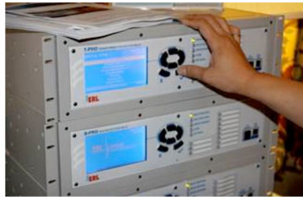
Above: 4000 series relays running IEC 61850 demonstration, using L-PRO Line Protection Relays.
