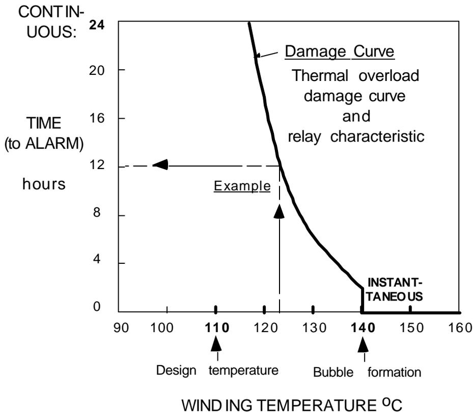
Fig. 3. Inverse time **overtemperature** protection.
