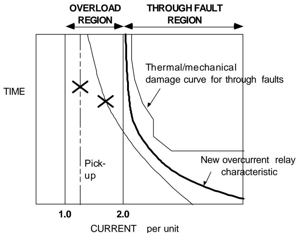
Fig. 2. Inverse time overcurrent **through-fault** protection.
