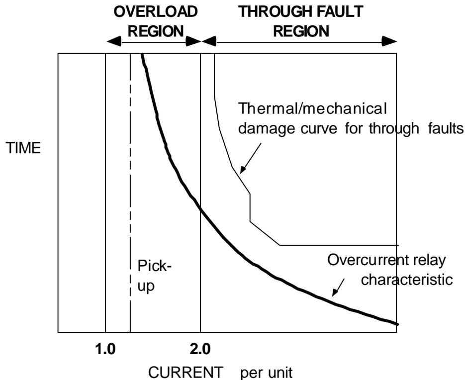
Fig. 1 Commonly used inverse time characteristic.
