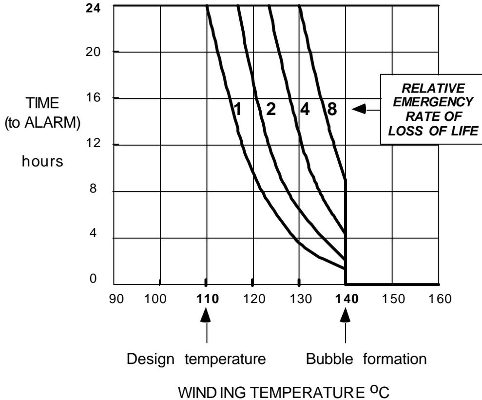
Fig. 4. Settings display for the **inverse time overtemperature** protection.
