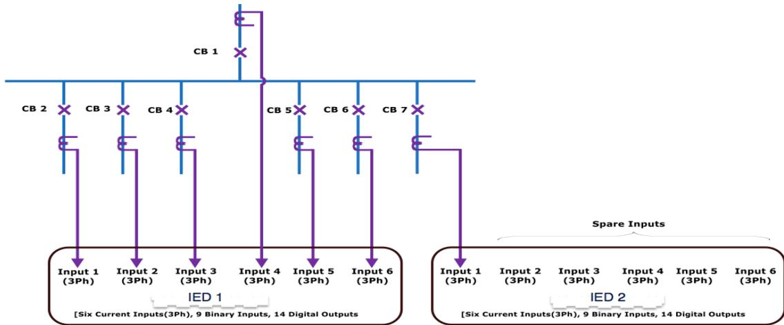
Figure 1: Illustrative 7 bays system with two IEDs for bus protection.
