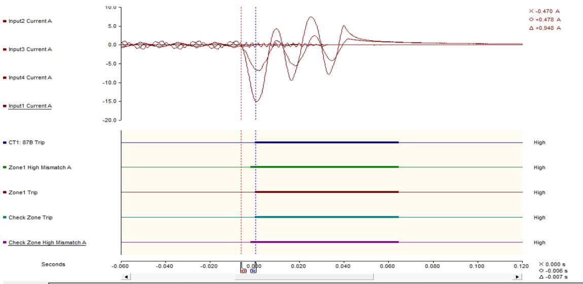
Figure 8: Transformer energization during an internal fault
