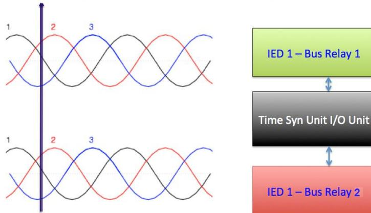
Figure 4: The time synchronization concept with two IEDs and an I/O unit
