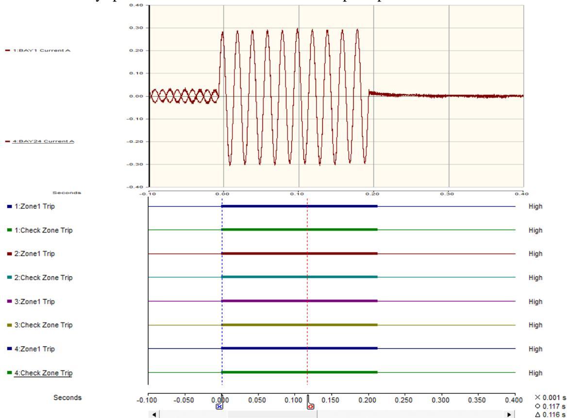
Figure 5: The 24 Bay differential protection operation within 9 milli-seconds after the fault inception.
