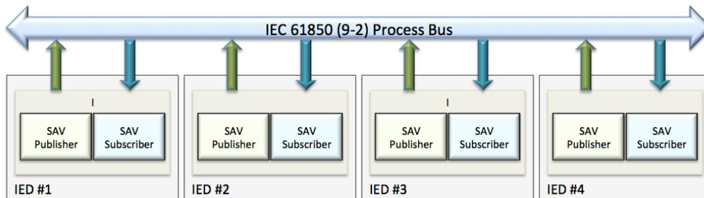
Figure 3: The sampled value (SAV) subscriber and publisher architecture used in each bus protection IED.
