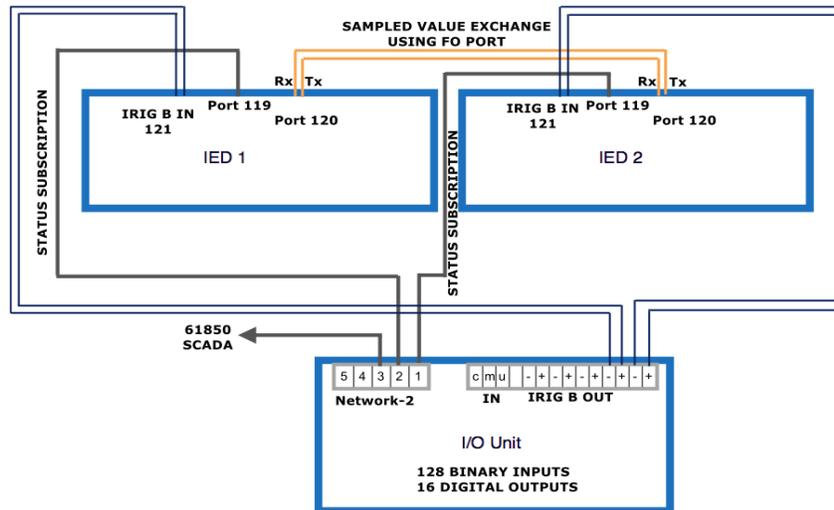
Figure 2: The network architecture for sampled value (9-2) and GOOSE (8-1) data exchange.
