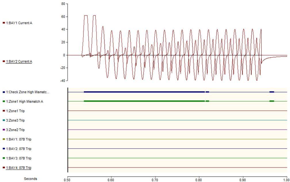
Figure 7: Extreme CT saturation with external fault.
