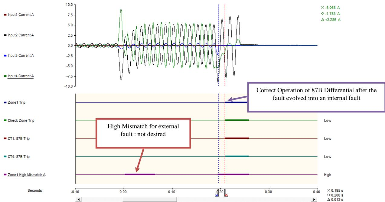
Figure 6: Evolving fault from external to internal bus zone.
