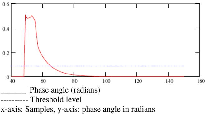
FIGURE 7: PHASE ANGLE ESTIMATION AND COMPARISON AGAINST THRESHOLD
