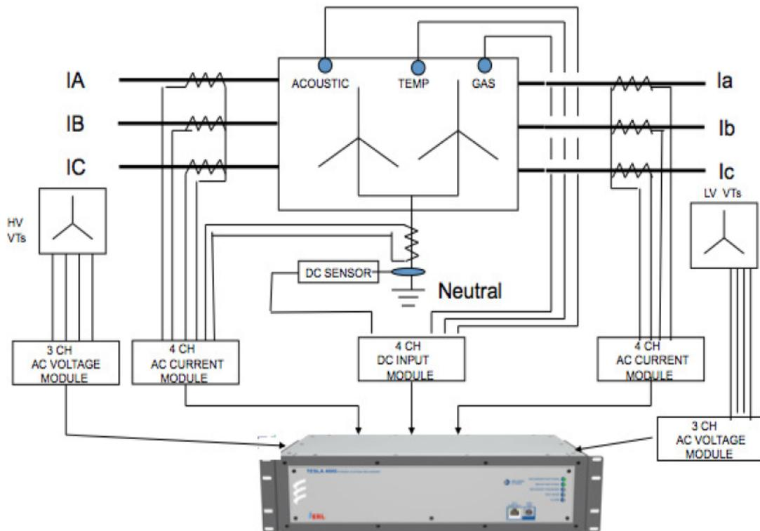
**Figure 7: Typical quantities measured by the GIC monitoring and detection device (TESLA DFR).**
