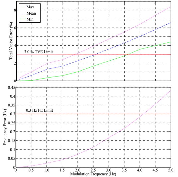
Fig. 8. TVE and FE response with modulation frequency at 60 fps without the performance class filters
