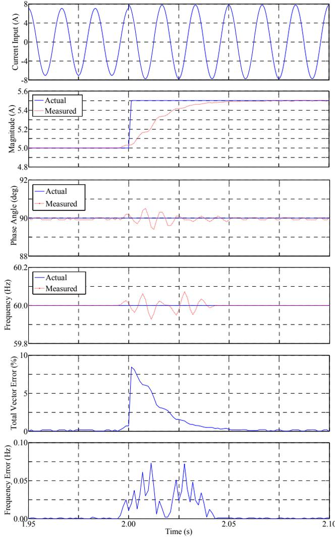
Fig. 11. Waveforms of magnitude positive step response at 60 fps Time response of the input signal, magnitude, phase angle, frequency, TVE and FE without the performance class filters ( $k_m = 10\%$  and  $k_a = 0\%$ )
