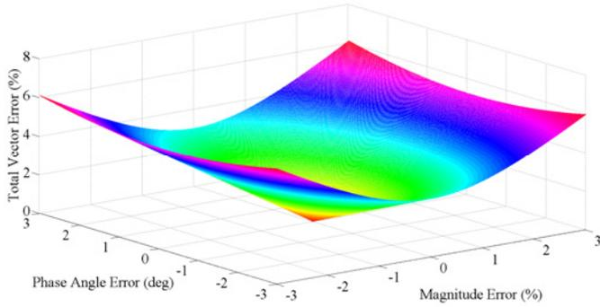
Fig. 2. TVE as a function of magnitude error and phase angle error
