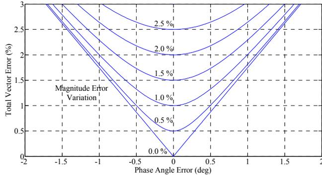
Fig. 3. TVE as a function of phase angle error for different magnitude errors
