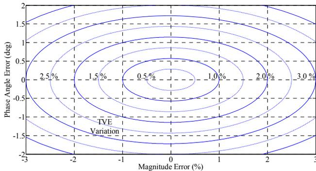
Fig. 5. Relationship between magnitude error and phase angle error for different TVEs
