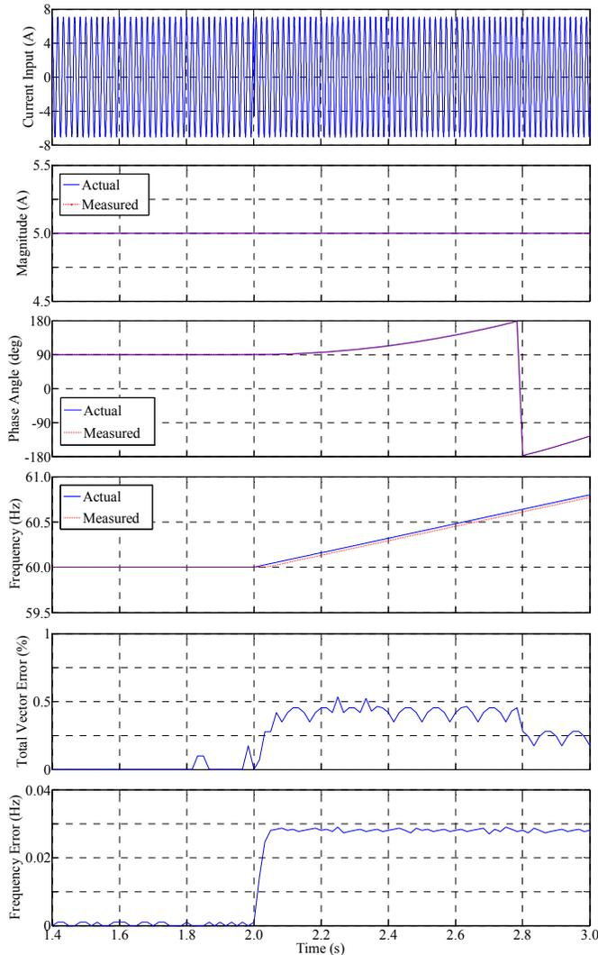
Fig. 9. Waveforms of linear frequency ramp response at 60 fps Time response of the input signal, magnitude, phase angle, frequency, TVE and FE without the performance class filters ( $R_f = 0.8$  Hz/s)
