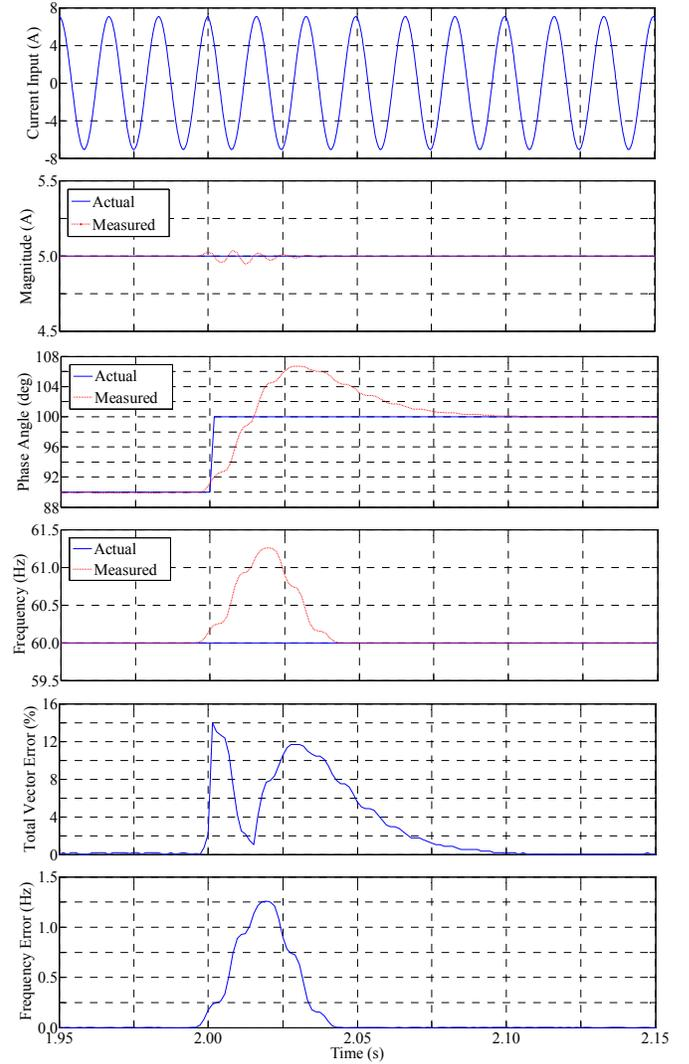
Fig. 12. Waveforms of phase angle positive step response at 60 fps Time response of the input signal, magnitude, phase angle, frequency, TVE and FE without the performance class filters ( $k_m = 0\%$  and  $k_a = 10\%$ )
