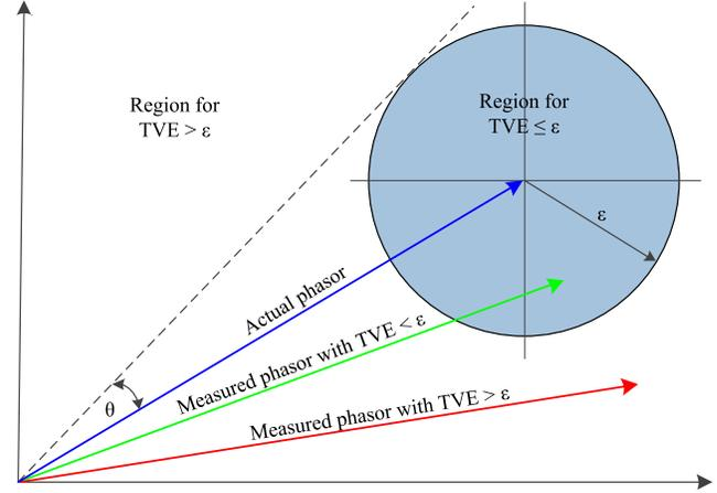
Fig. 1. Relationship between actual phasor, measured phasor and TVE
