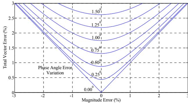
Fig. 4. TVE as a function of magnitude error for different phase angle errors
