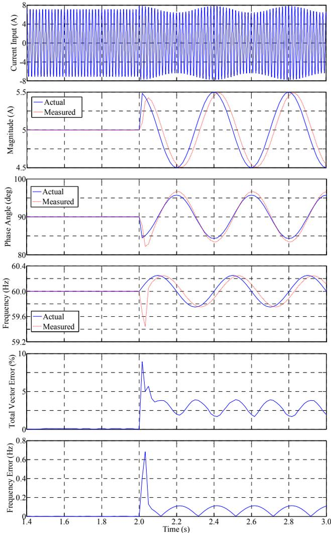
Fig. 7. Waveforms of measurement bandwidth response at 60 fps
