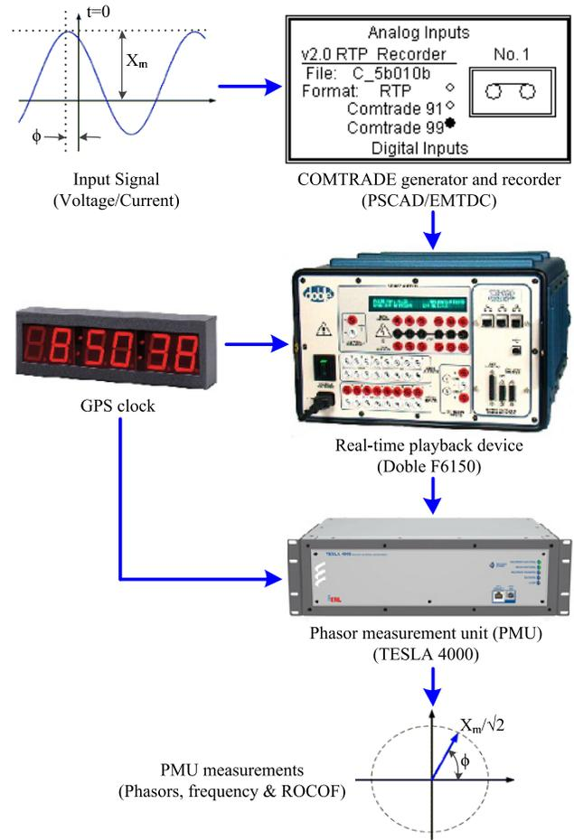
Fig. 6. Operational flowchart of test setup
