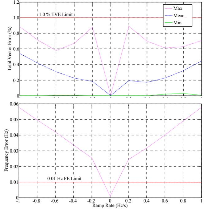
Fig. 10. TVE and FE response with linear frequency ramp at 60 fps without the performance class filters
