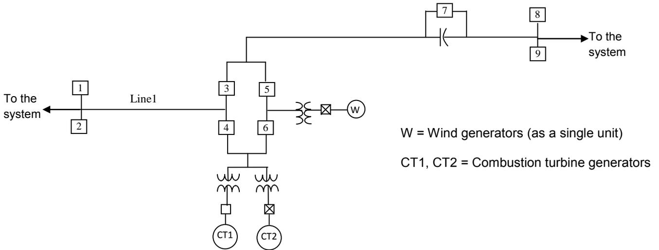
Figure 1: System one line diagram – All breakers were closed except CT1 breaker and Breaker-7.
