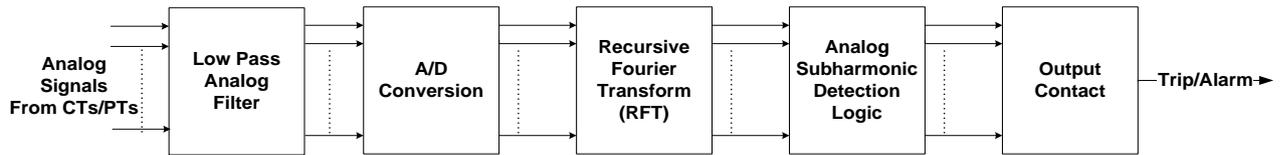
Figure 4: Illustration of the sub-harmonic detection process.
