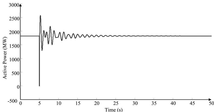
**Fig. 8** Active power output of generator 16 subsequent to a contingency**Table 8** Mode parameter estimations: 50-generator 470-bus test system
