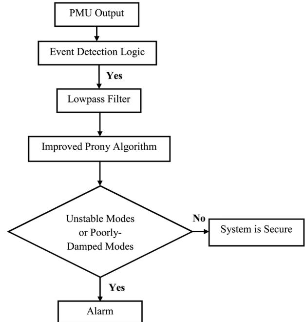
Fig. 4 Proposed oscillation monitoring algorithm
