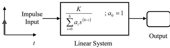
Fig. 2 Test linear system
