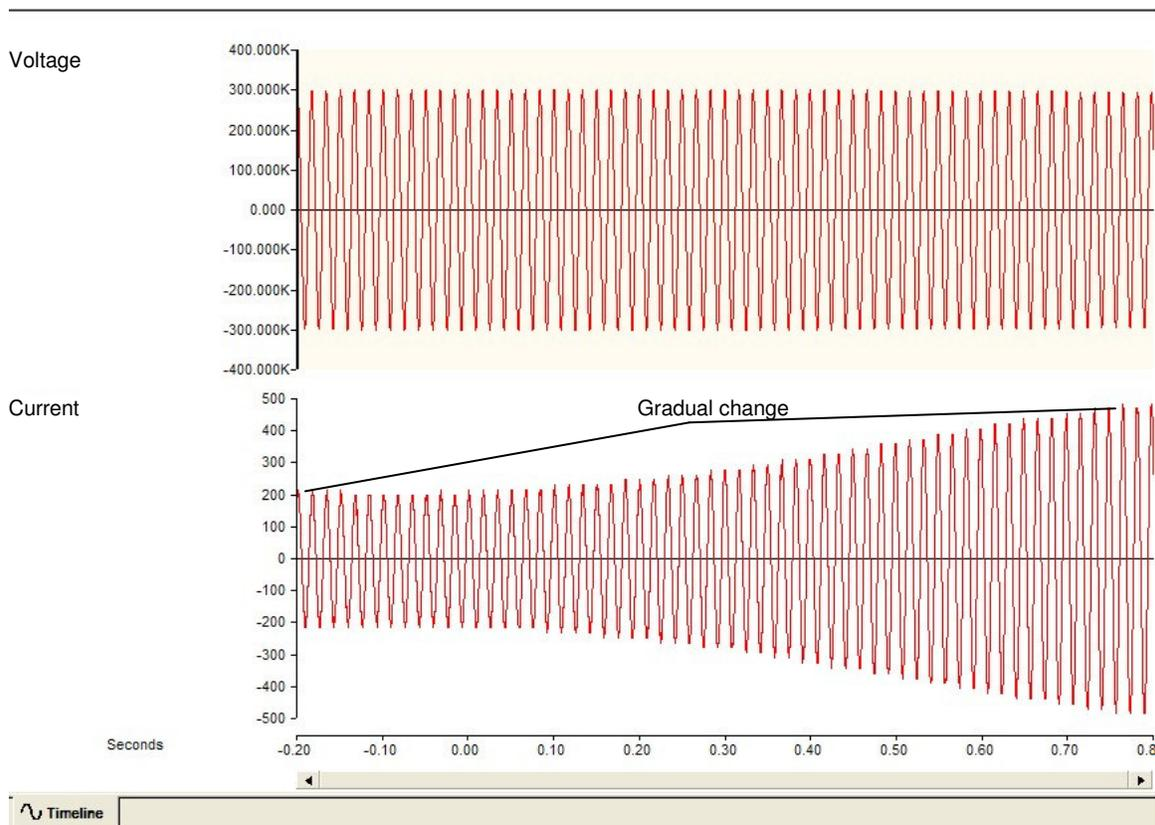
**Figure 4: Power system fault – speed of fault inception**
