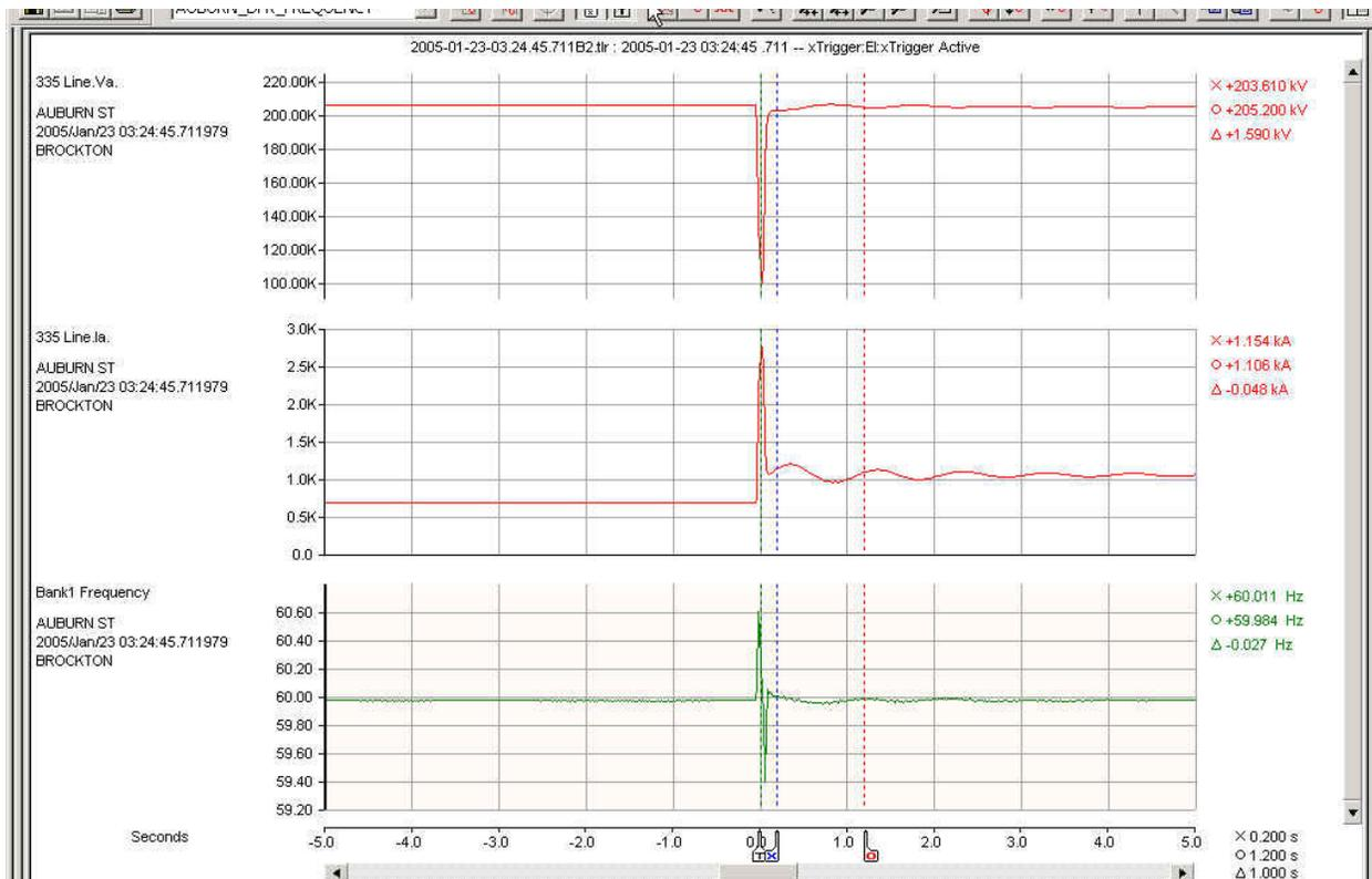
**Figure 6: Voltage and Current quantities from power equipment fault**
