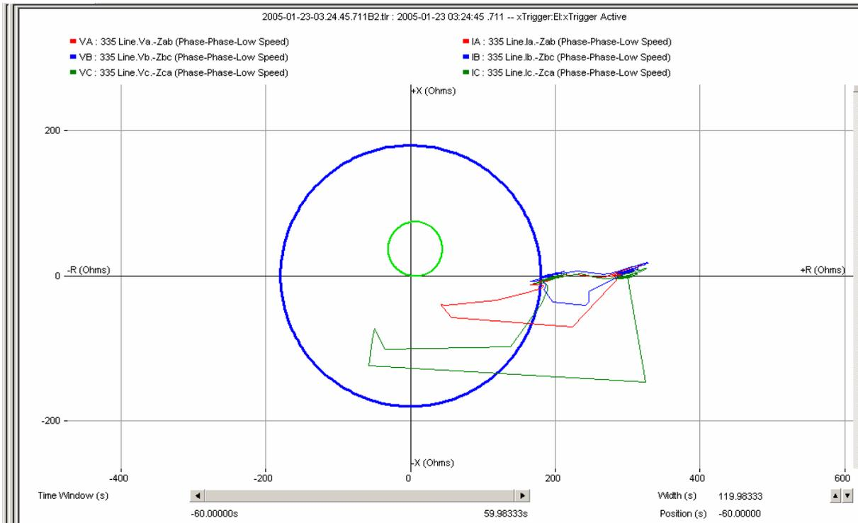
**Figure 8: Impedance trigger for local fault event**
