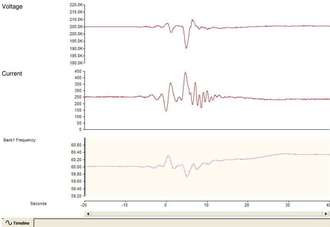
**Figure 2: Power system fault (swing) record**
