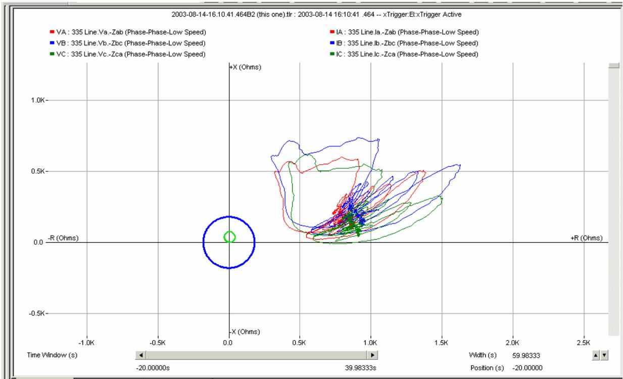
**Figure 7: Impedance trigger for power swing event**
