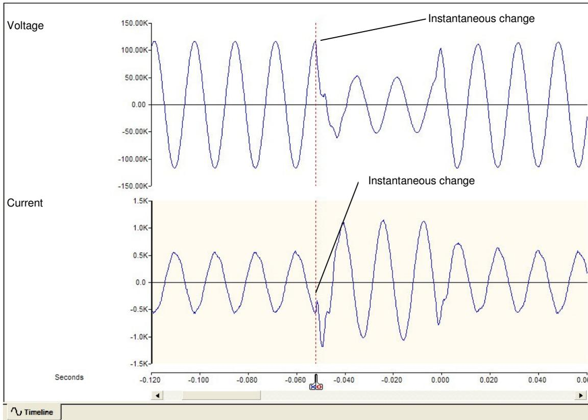
**Figure 3: Power equipment fault – speed of fault inception**
