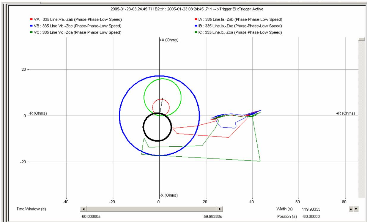
**Figure 9: Impedance trigger for protection system verification**
