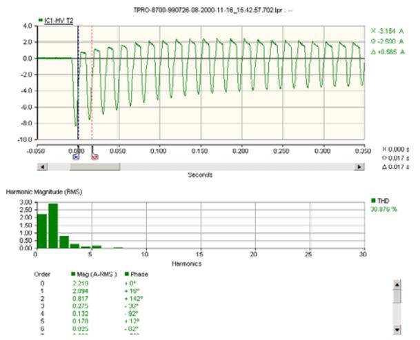
**Fig-6c: Record and harmonic spectrum for a typical inrush current at phase C of the transformer**
