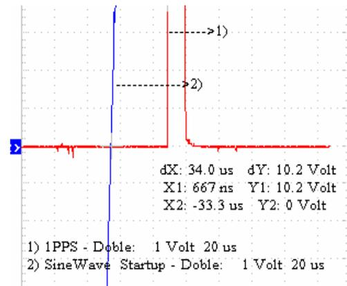
a) SinWave startup with respect to 1PPS – Manufacturer A
