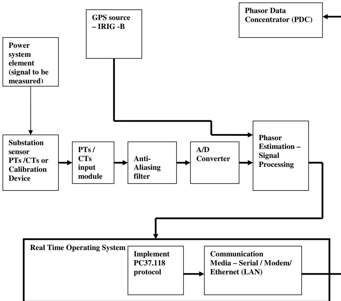
FIGURE 2: PHASOR ESTIMATION AND POSSIBLE SOURCES OF ERRORS
