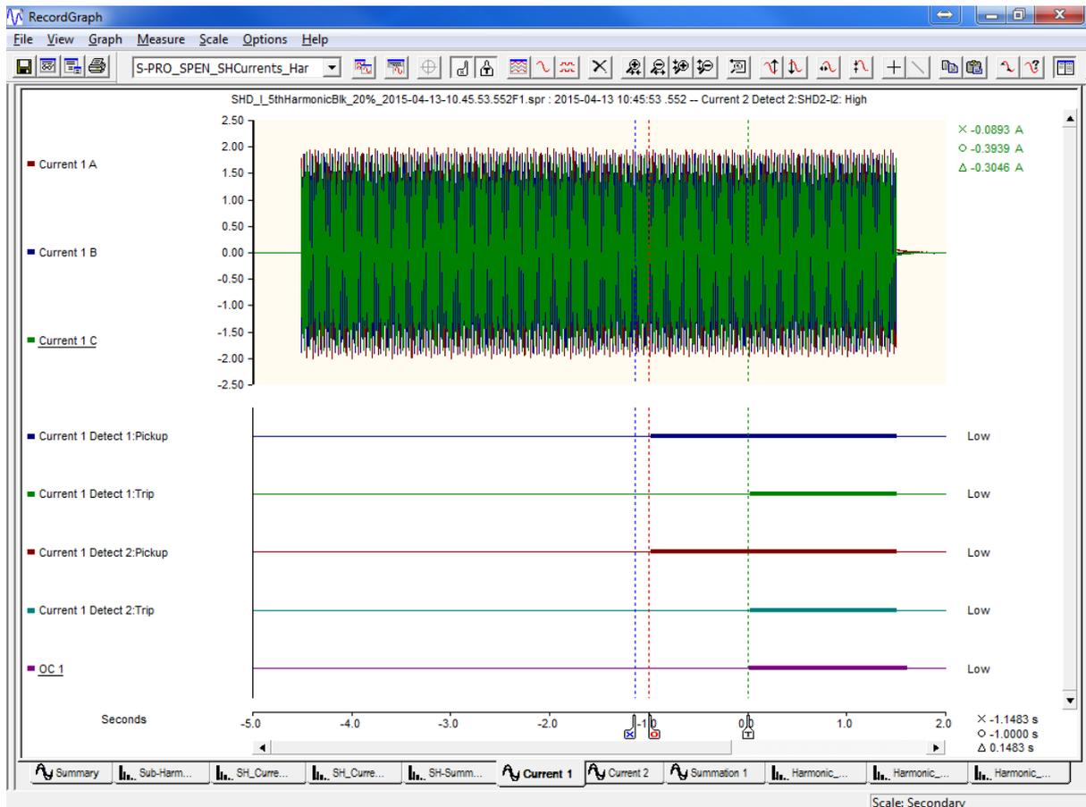
Figure 16 - Relay Operation in response to 2nd or 5th Harmonics
