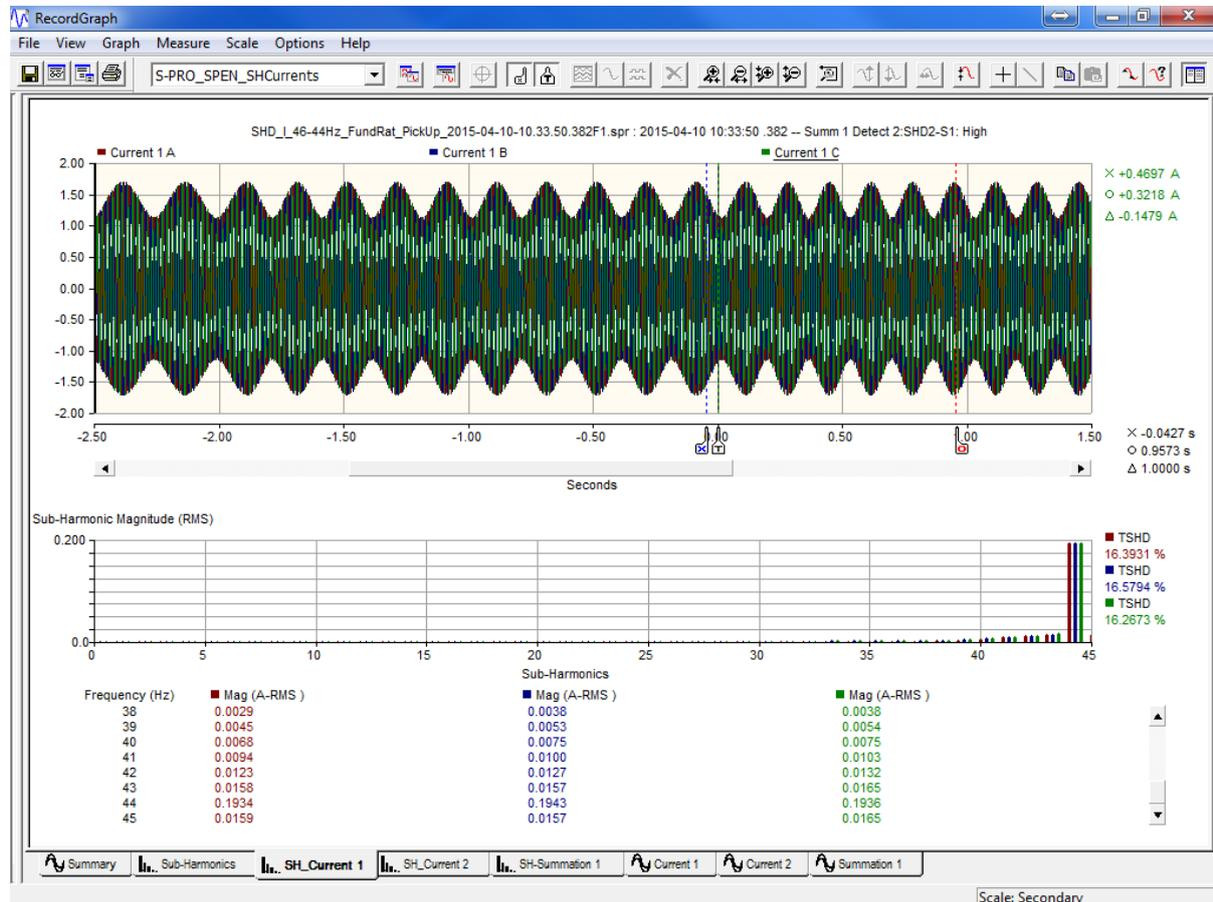
Figure 7 - Current Waveform used to test Maximum Frequency
