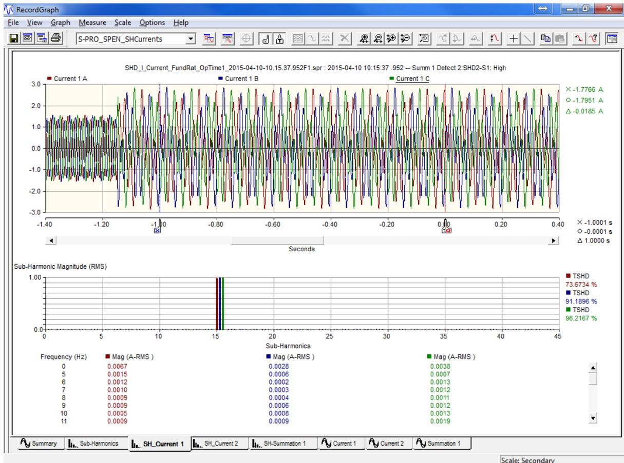
Figure 11 - Waveform used to test Relay Operating Time
