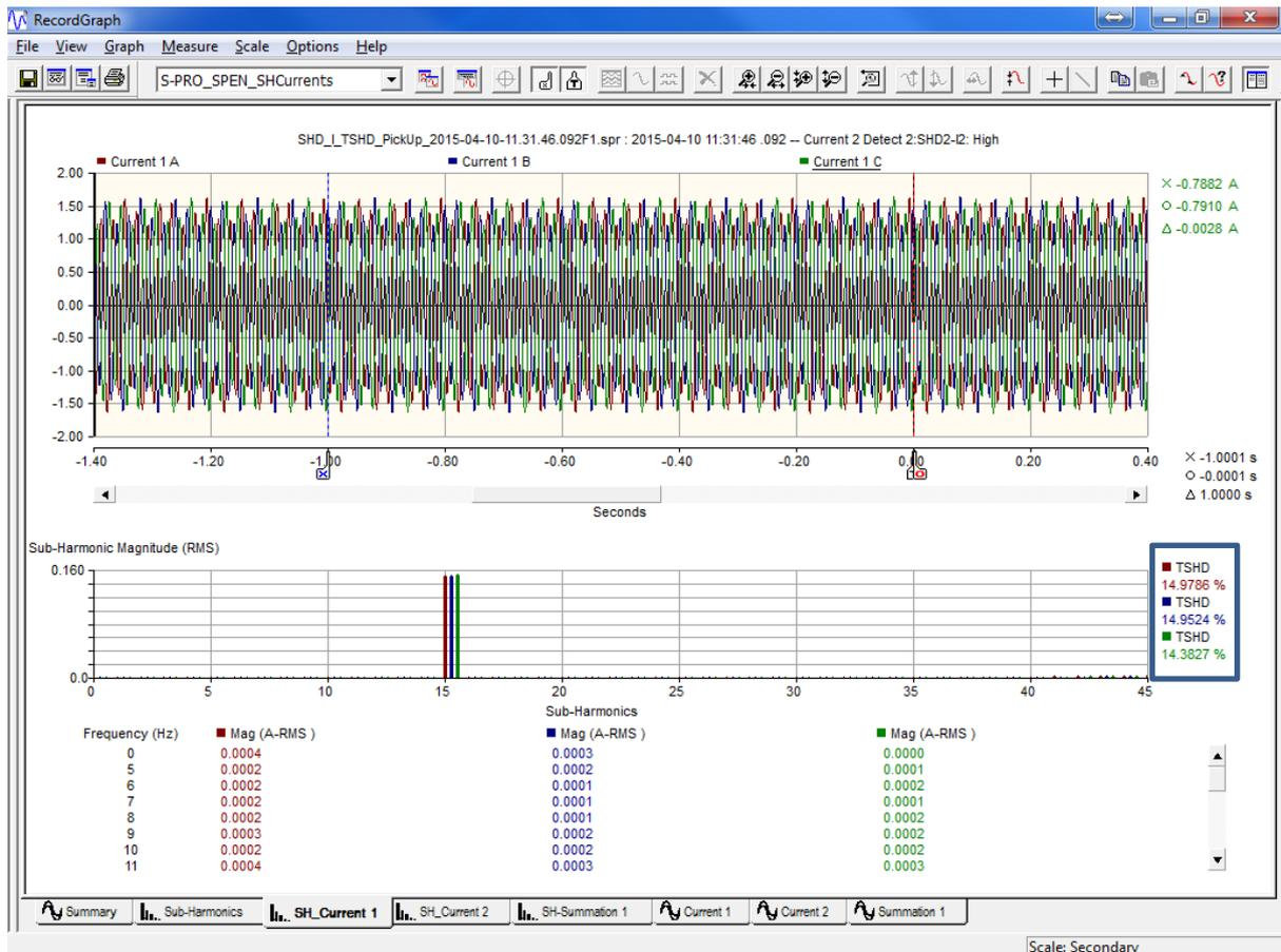
Figure 9 - Current Waveform used to test Total Sub-harmonic Distortion (TSHD)
