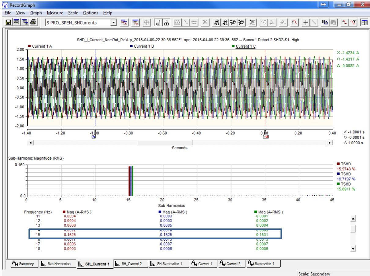
Figure 8 - Current Waveform used to test Nominal or Fundamental Ratio Pickup
