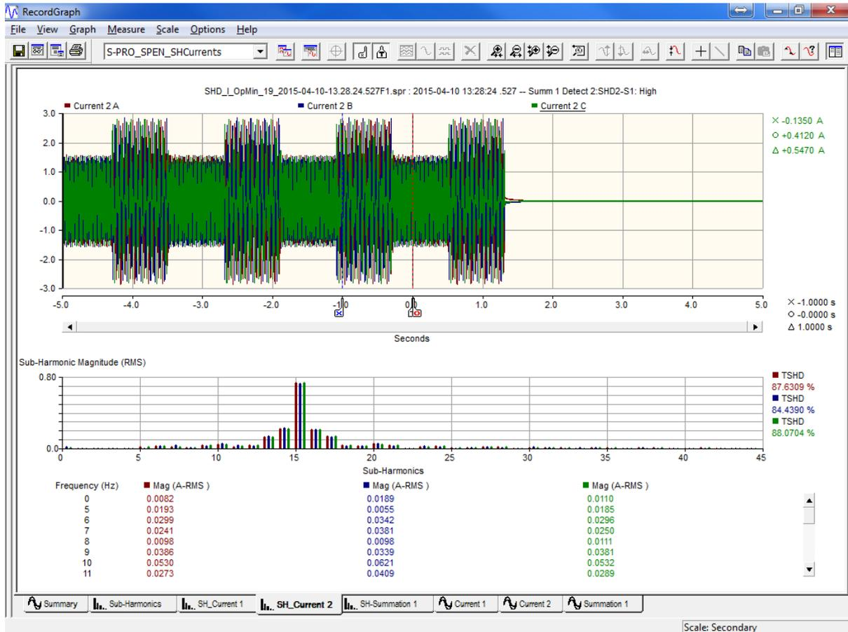
Figure 13 - Waveform used to test Operations per Minute
