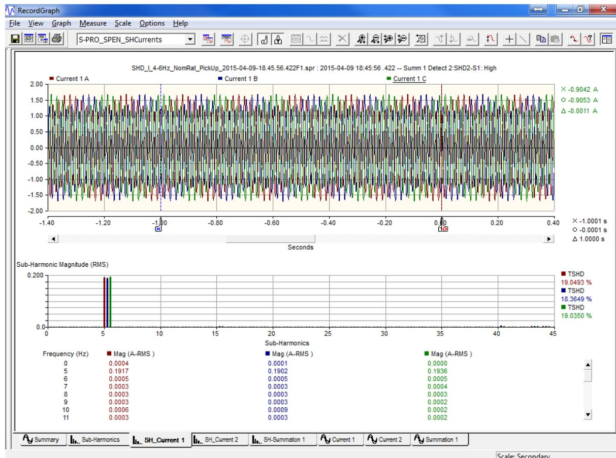
Figure 6 - Current Waveform used to test Minimum Frequency
