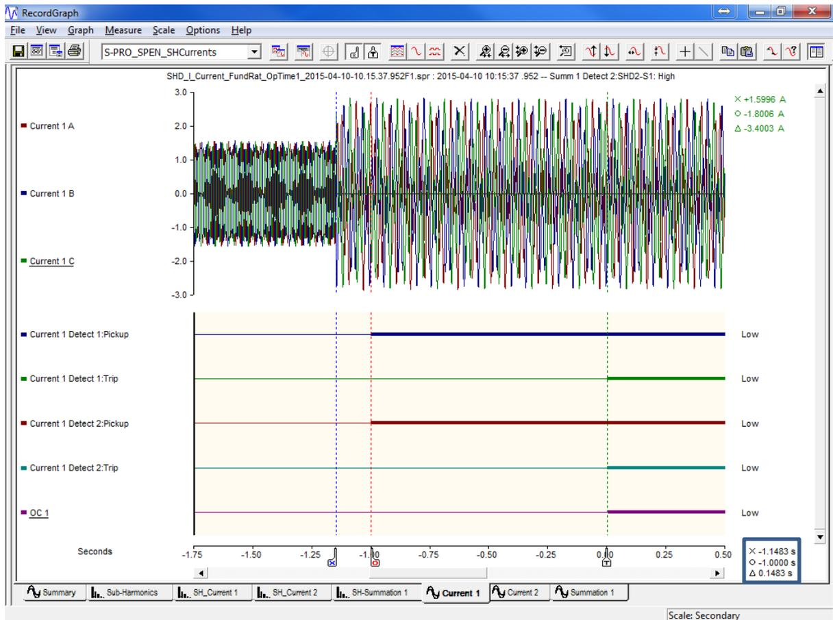
Figure 10 – Relay Operating Time
