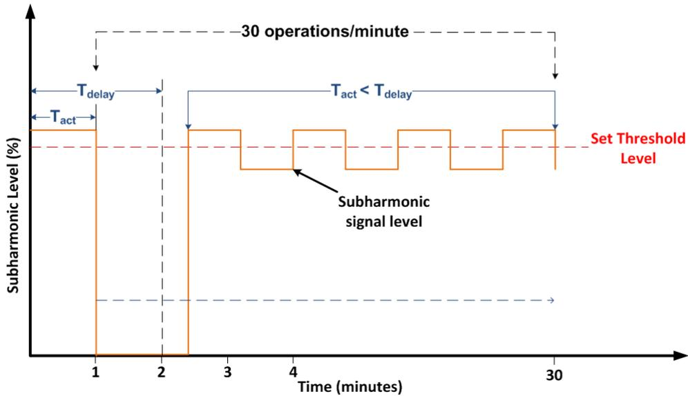
Figure 4 - Operations per minute principle
