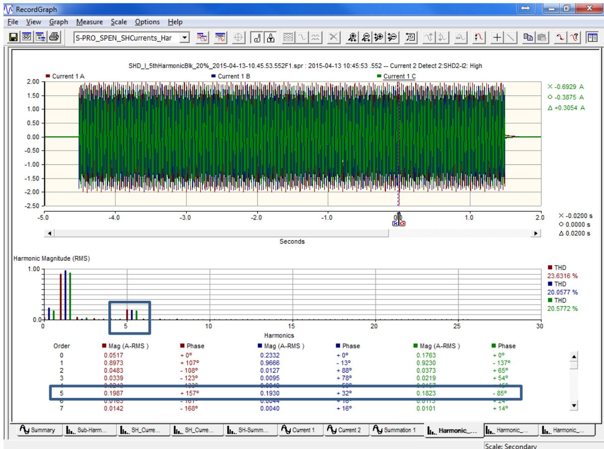
Figure 15 - Waveform used to test 5th Harmonic Blocking
