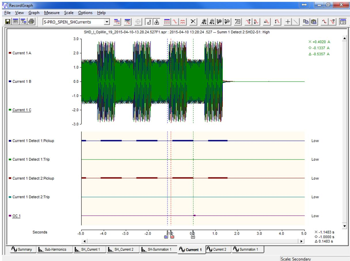
Figure 12 - Relay Response for Operations per Minute
