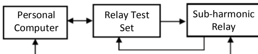
Figure 5 - Equipment Setup for Testing
