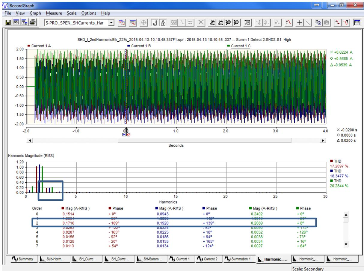
Figure 14 - Waveform used to test 2nd Harmonic Blocking
