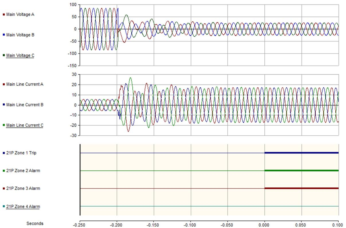
Figure 11: Zone mis-operation during reverse faults (no-modified algorithm)
