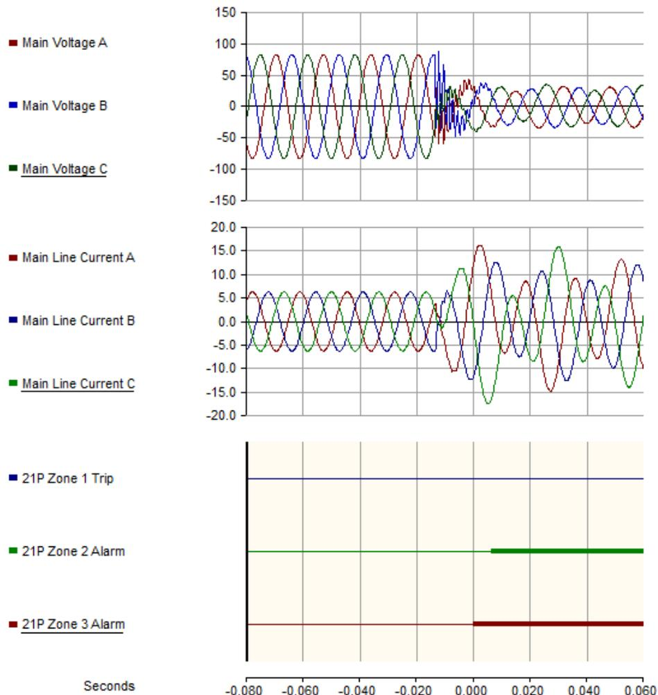
Figure 8: Overcoming zone-1 over-reach due to sub-harmonics (modified algorithm)
