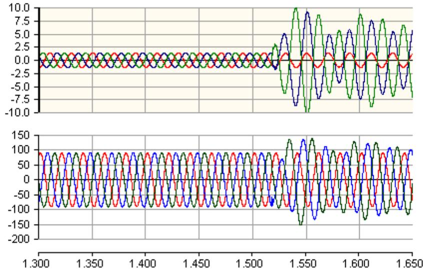
Figure 2: Typical sub-harmonic waveform [11]
