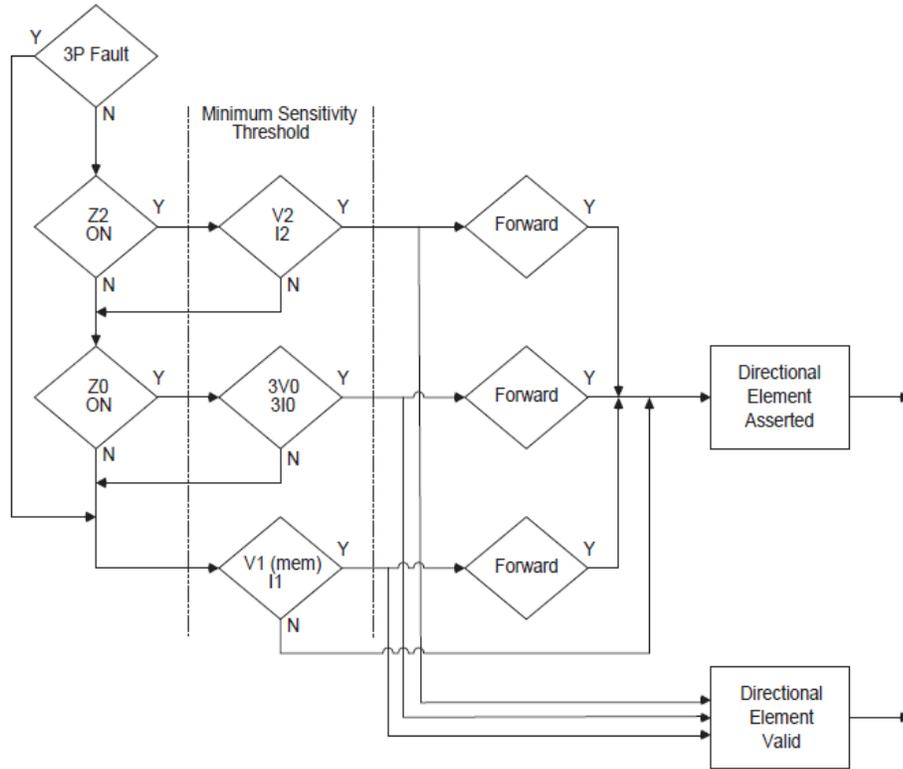
Figure 3: Directional element logic
