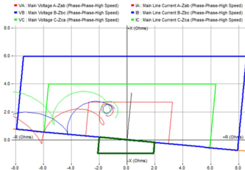
Figure 1: Mis-operation of distance relay during voltage inversion
