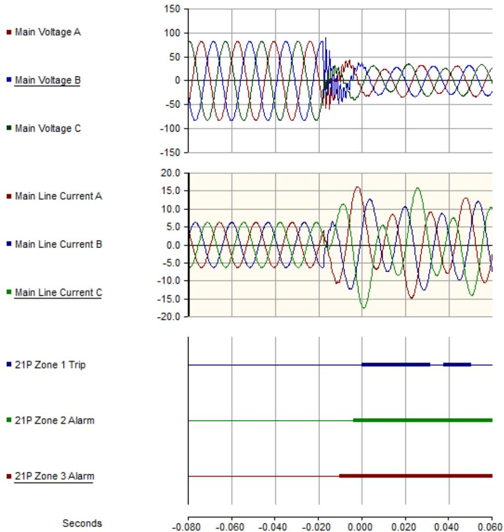
Figure 9: Zone-1 over-reach due to sub harmonics (no-modified algorithm)
