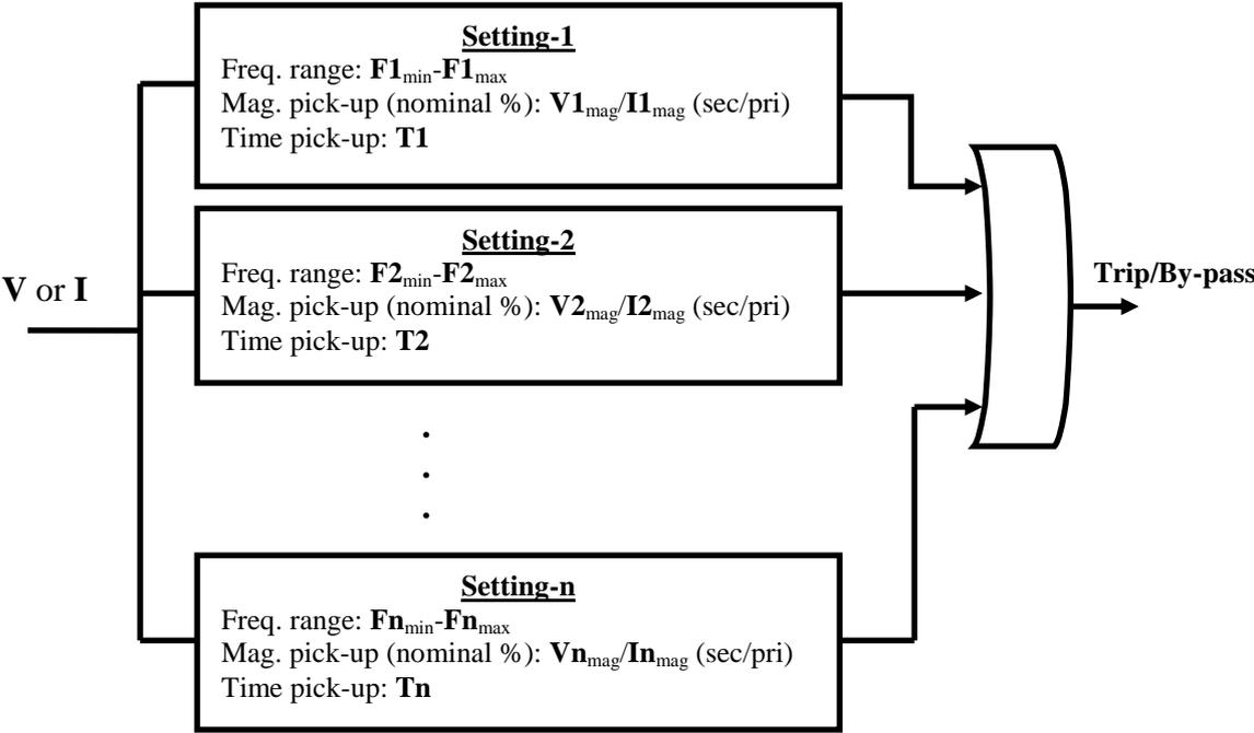
Fig. 4. Proposed Protection Logic
