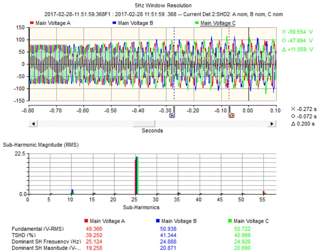
Fig. 7. Sub-harmonic spectrum of voltage signals
