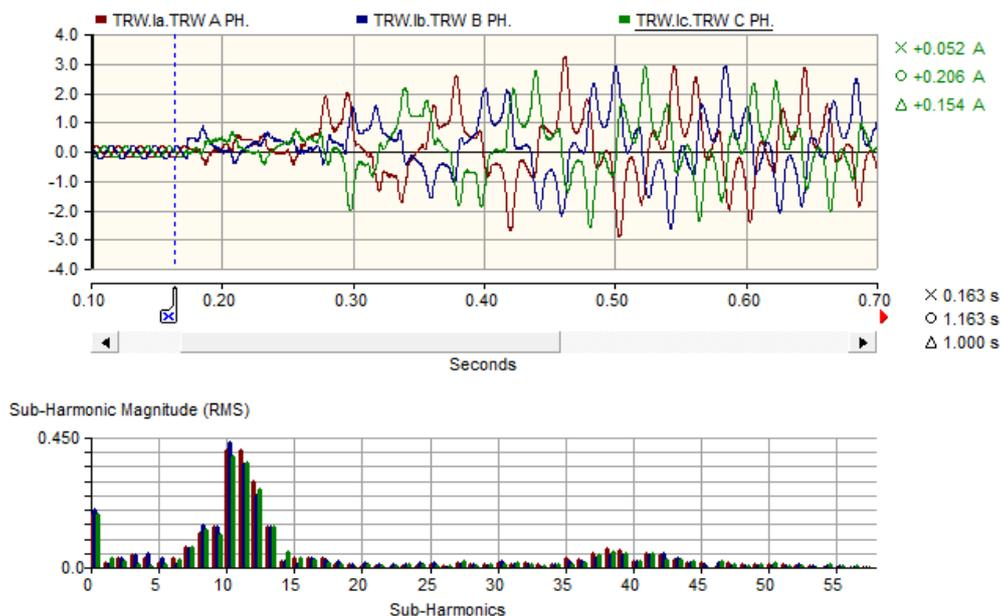
Fig. 1. Field recorded waveform during a SSO condition
