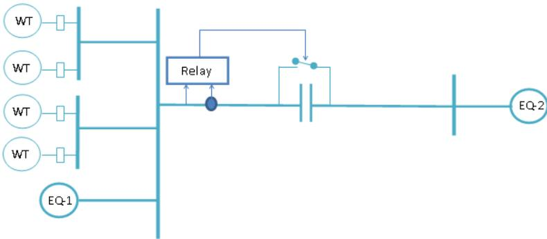
Fig. 2. Relay arrangement for by-passing the series capacitor
