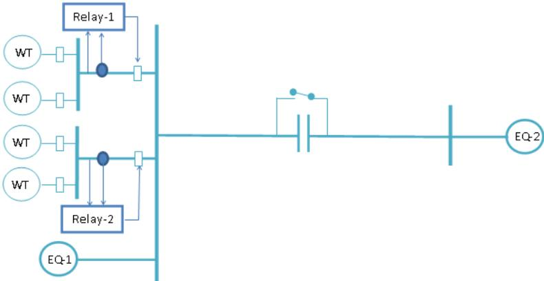
Fig. 3. Relay arrangement for tripping the windfarm
