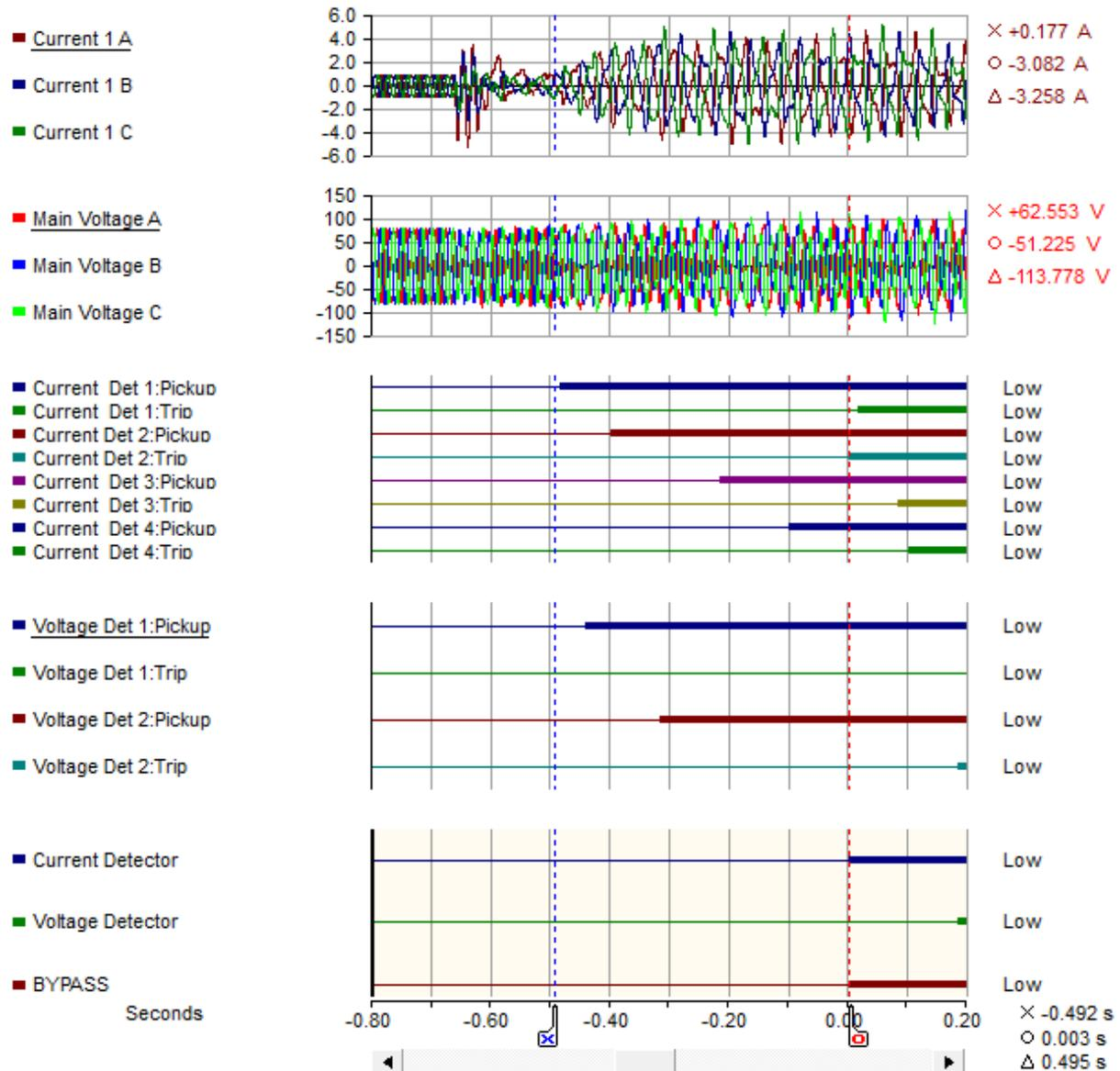
Fig. 5. Operation of the relay
