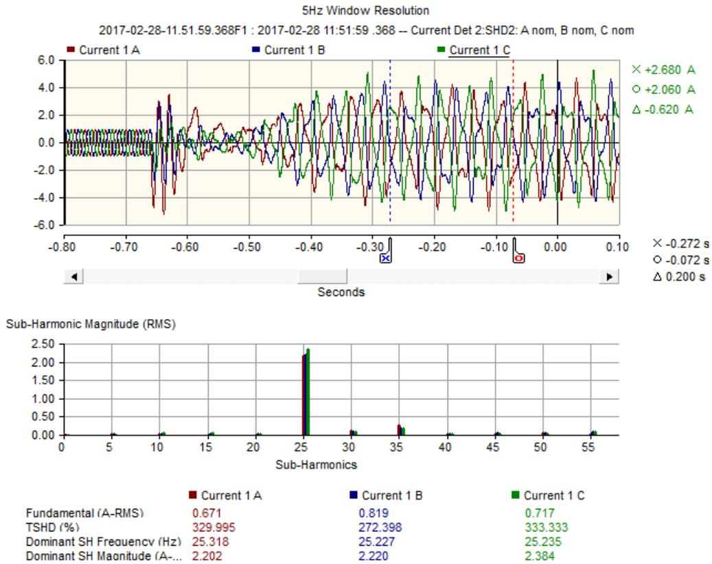
Fig. 6. Sub-harmonic spectrum of current signals
